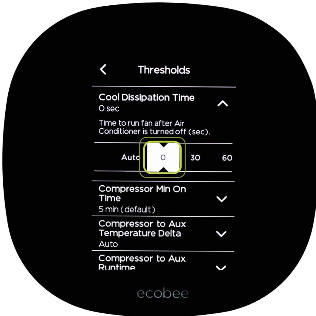
This maximizes the amount of humidity removed during cooling mode.
