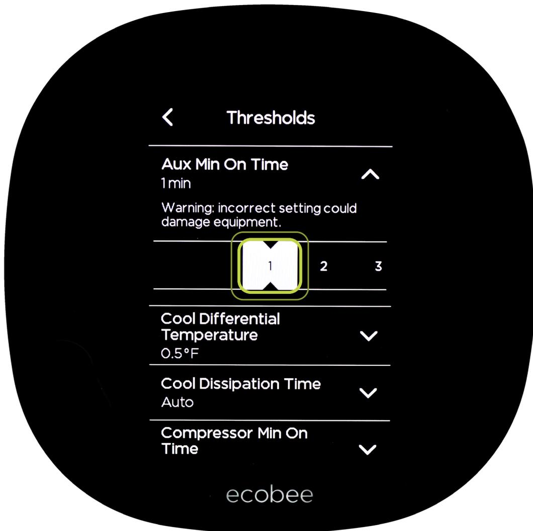
This setting regulates the electric heat runtime, which maximizes energy savings and increases system durability.
