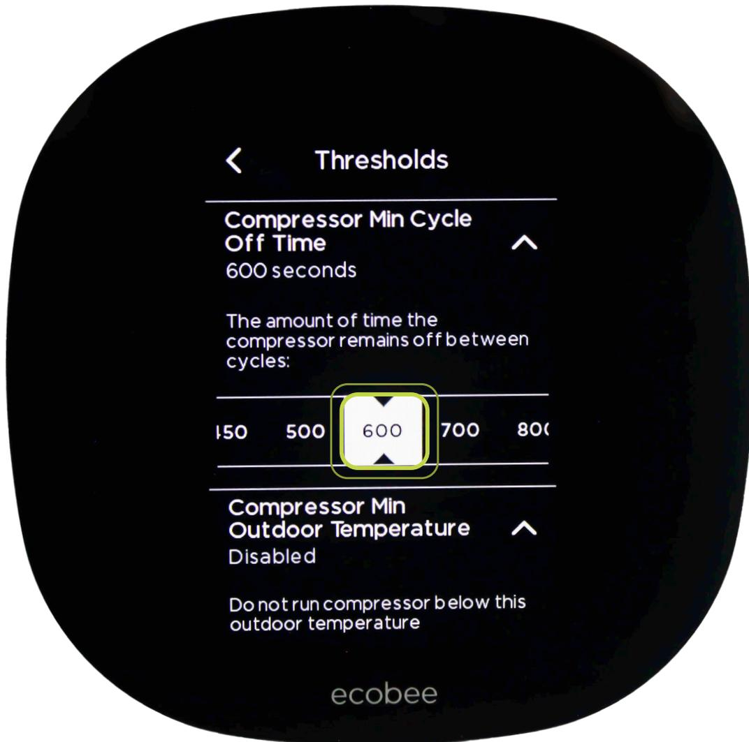
This is a recommended setting to save energy and increase equipment durability. After the unit cycles off, it will not come back on for 10 minutes.
