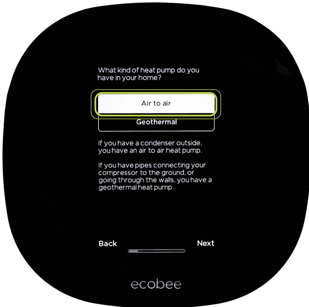
These are the recommended settings for an all-electric air to air heat pump. See the ecobee SmartThermostat installation documents if any other source of heating (geothermal, furnace, etc.) is present.
