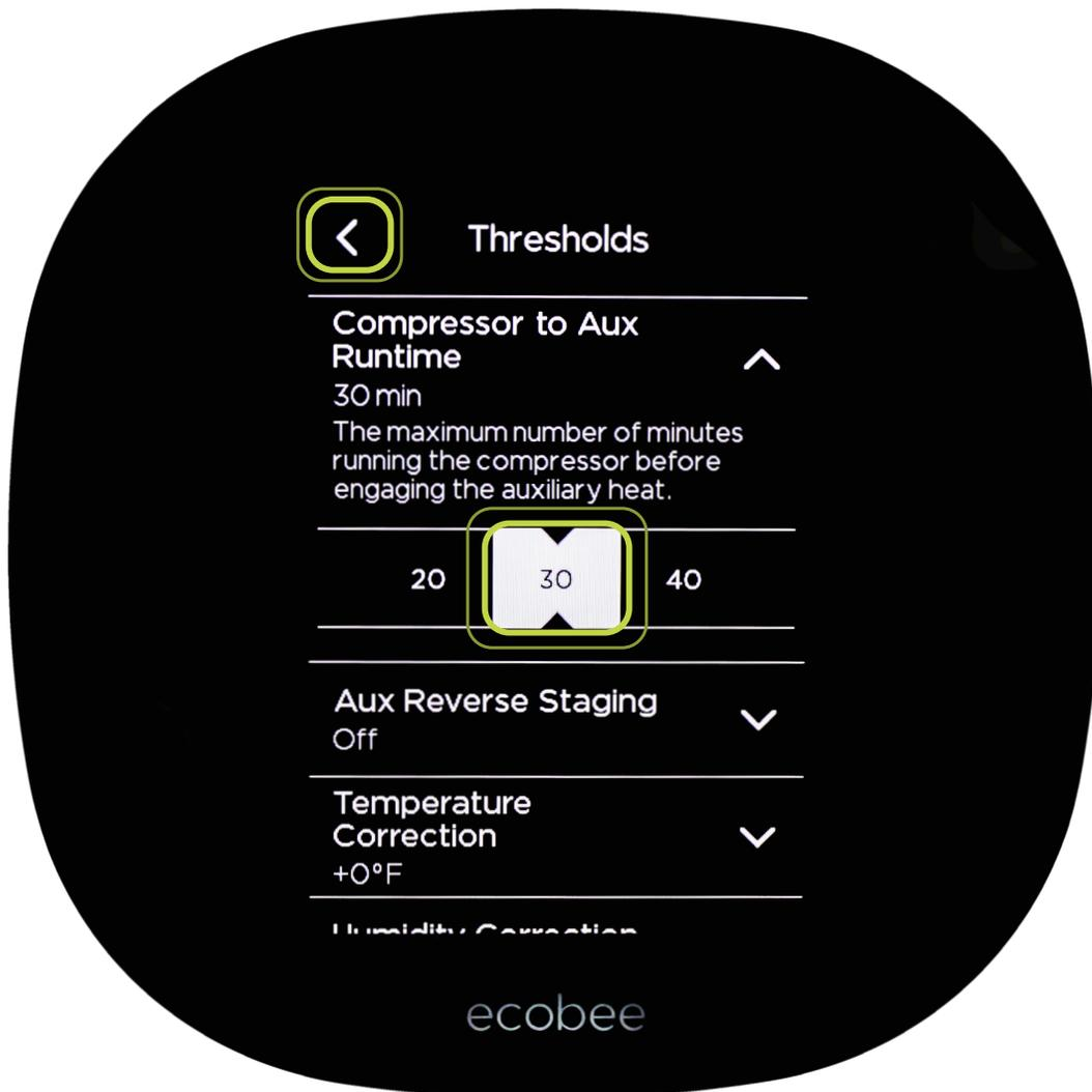
This is to maximize the efficiency of your air source heat pump before less efficient strip heat comes on to maintain comfort at lower temperatures.
